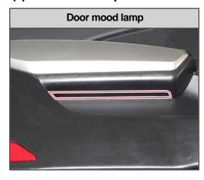
The door mood lamp comes on when the tail lamp switch is operated.
