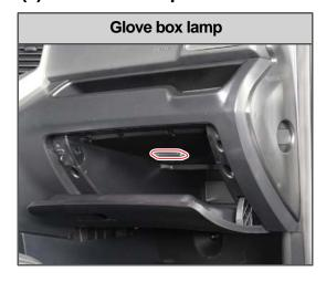
The glove box lamp comes on when the glove box is opened after the tail lamp switch is operated.
