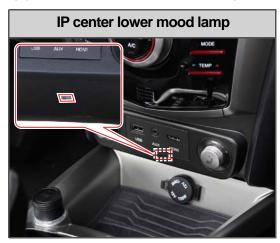
The IP center lower mood lamp comes on when the tail lamp switch is operated.
